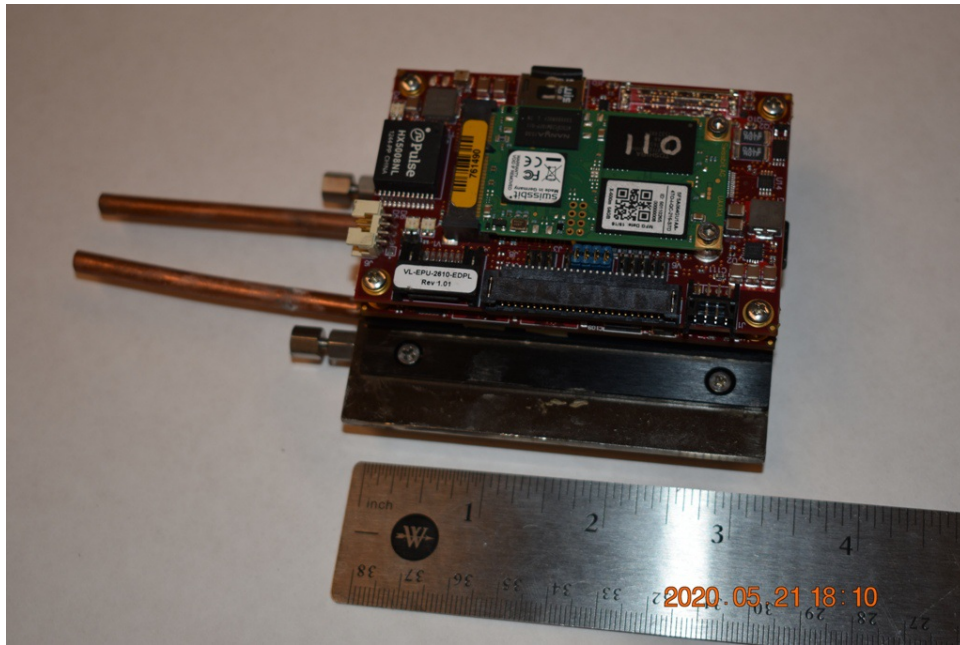
Photo 1: two copper tubes sticking out of the heat sink are the heat pipes that connect said heat sink to the external cooling fins.
